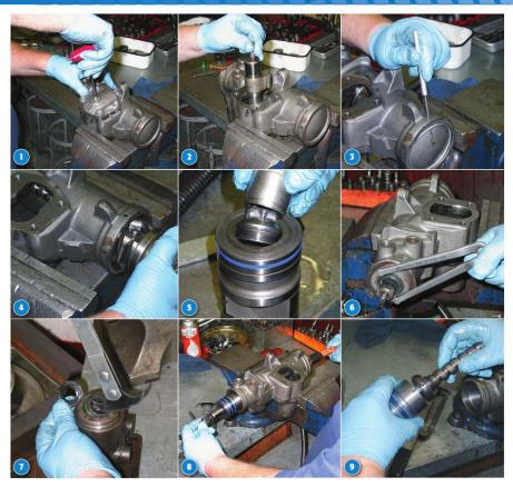
1 With the box out of the car, clean the case thoroughly. Disassembly begins by pulling the Pitman arm off with a puller-no pickle fork or hammer because they'll damage your case. Up top is the side cover. Remove its four bolts, then use an Allen wrench to turn the adjuster counter-clockwise and remove the side cover.
