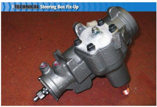
It wasn't just QuadraJet carbs that Ford has sourced from GM. This 1971-'73 Mustang integral steering box is built by Saginaw, a GM division. Internally, they are the same, but the cases have different mounting points, so they are not interchangeable. Used in most of the high-volume musclecars of the '60s, there are lots of service parts available for them, including a slick conversion to a quicker 12:1 ratio.
