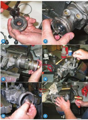
16 The bearing is installed into the adjuster/retainer with a press, then the O-ring and seals are installed and held in place with a snap ring. The bearing and seals are lubed, then the adjuster/retainer is carefully slipped over the input shaft and threaded into the case.
