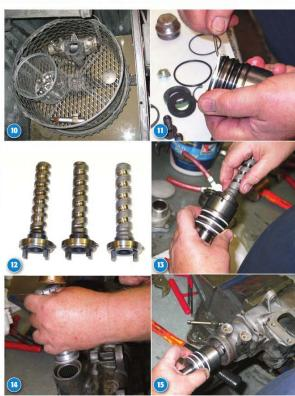
10 With all the seals, washers, bearings, and other parts out of the case, all the parts to be reused will go into a strong hot detergent bath. Then, they spend some quality time in the parts washer. Some get a cleanup on the wire wheel, and the castings are carefully checked for cracks and heavy wear that will require more than a light hone. Heavy wear means using a replacement part from a core or sleeving the cylinder.
